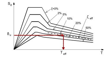
• Calculate the effective stiffness of the substitute structure:
