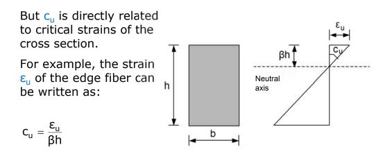
Thus, the ultimate displacement,  $\delta_{\rm u},$  can be associated with the critical strains of the cross section of the plastic hinge.
