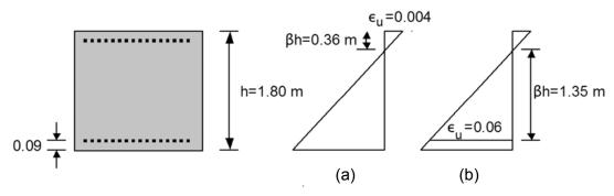
a) If the critical check concerns the compression of the concrete: Let max $\epsilon_u$  = 4‰. Also,  $\beta$ h = 0.36 m,  $\beta$  = 0.36/1.80 = 0.2.  $\frac{\delta_u}{L} = \frac{0.004}{0.2 \times 2} = 0.01$
